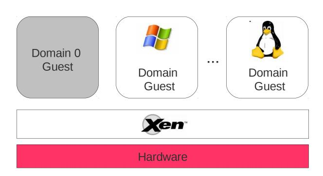
The **Xen hyperviso**r runs directly on the hardware and becomes the interface for all hardware requests such as CPU, I/O, and disk for the guest operating systems. By separating the guests from the hardware, the Xen hypervisor is able to run multiple operating systems securely and independently.
